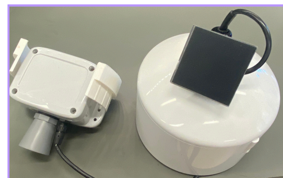
Figure 2 : The exterior of the Flood sensor. The Flood sensors are usually placed outside in capsules to prevent damage to them. The cap on the right is the cover to the tube and the system is powered with the solar cell on top.
